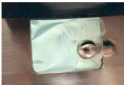
Figure 7. BPC tab holders used for proper BPC positioning
