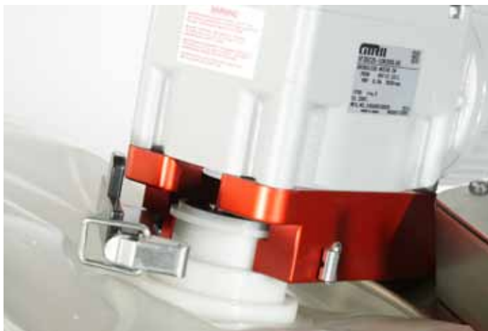
Figure 6. Bearing port inserted into motor mount slot and clamp
