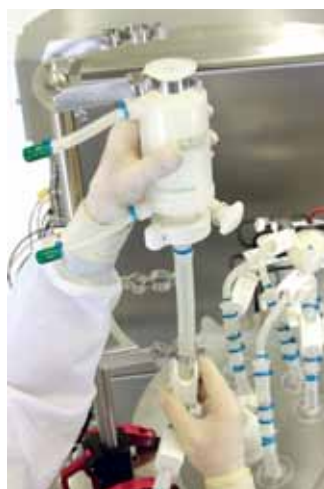
Figure 8. Filter being placed in bracket
